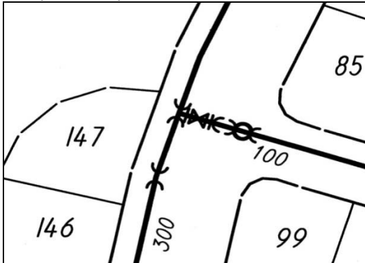
Sample 1: Stop valve in branch water main
