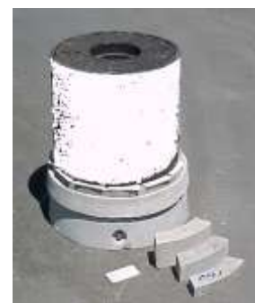
Concrete Fibre Cement (may contain Asbestos)
