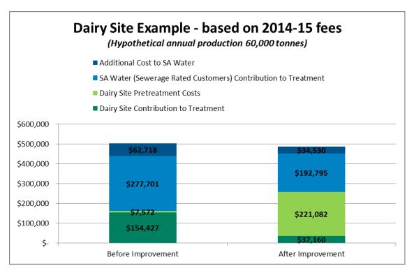
The dairy site example shows that with the installation of a DAF system, the overall annual cost associated with the site's trade waste discharge marginally decreased, but significantly reduced the cost to SA Water and sewer rate paying customers. The key points are:
