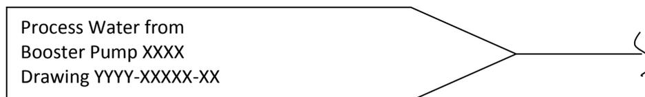
Figure 1 - Typical process flow tag format for incoming process flow (left of page)
