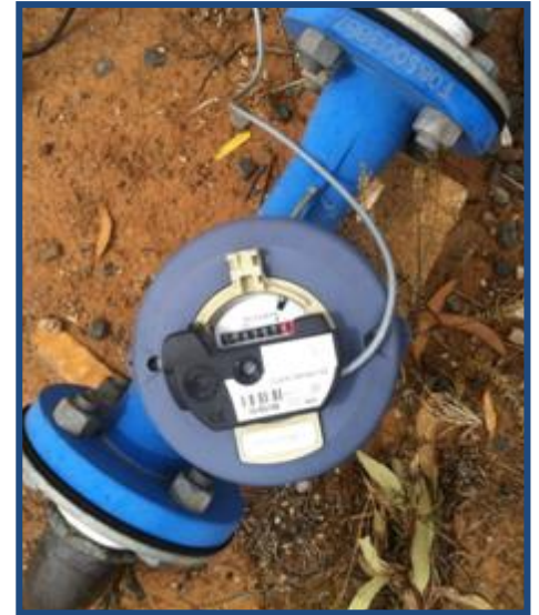
Figure 1: Data logging sensor on a meter
