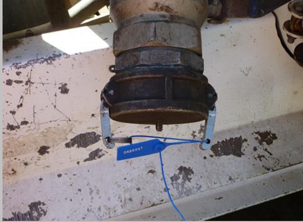
Figure 1: A tamper proof seal attached to the cam-lock cap of a trucks outlet
