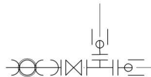
Figure 9: Cutout of the existing main – flanged tee with gibaults
