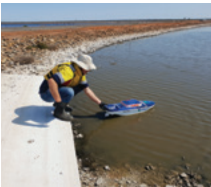
One of the new remote-controlled boats now being used to survey sludge lagoons.
