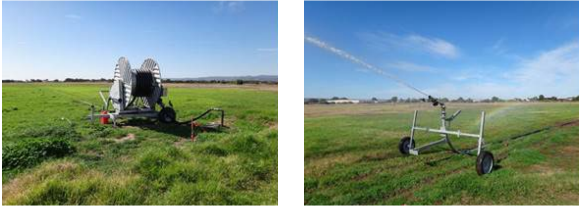
Figure 2. Showing the cannon and reel components of the irrigation system
