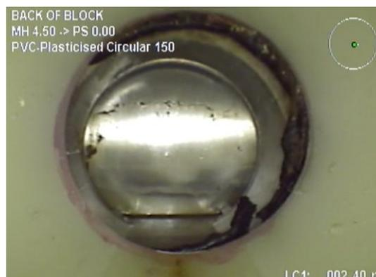
**Figure 11 Excessive Solvent Cement**
