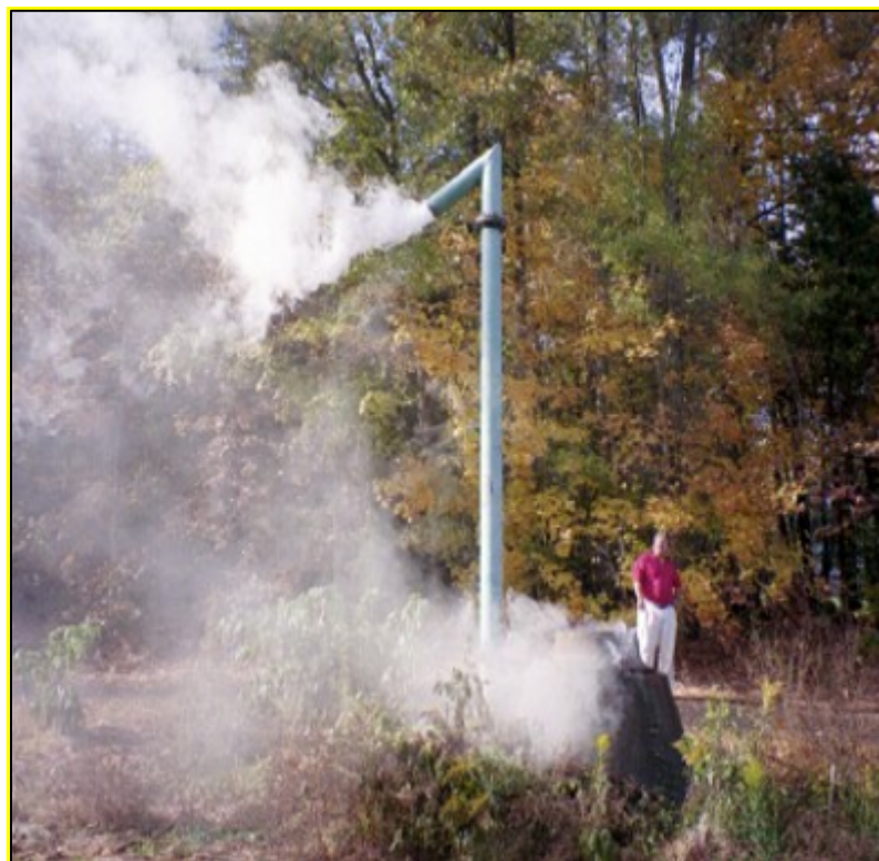
Figure 12: Uncontrolled air release caused by hydraulic surge
