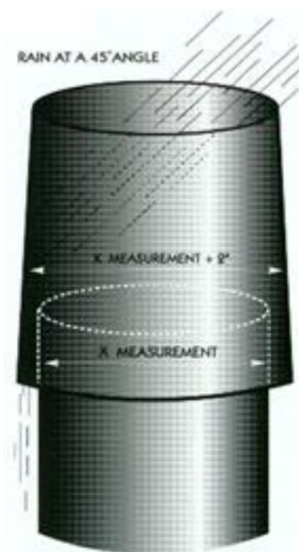
Figure 23: Collar-type rain guard for a stack
