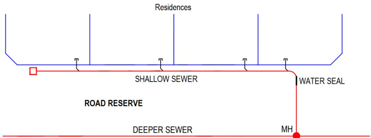
**Figure 11-1 Connection of residences to a trunk sewer via reticulation sewer with water seal**
