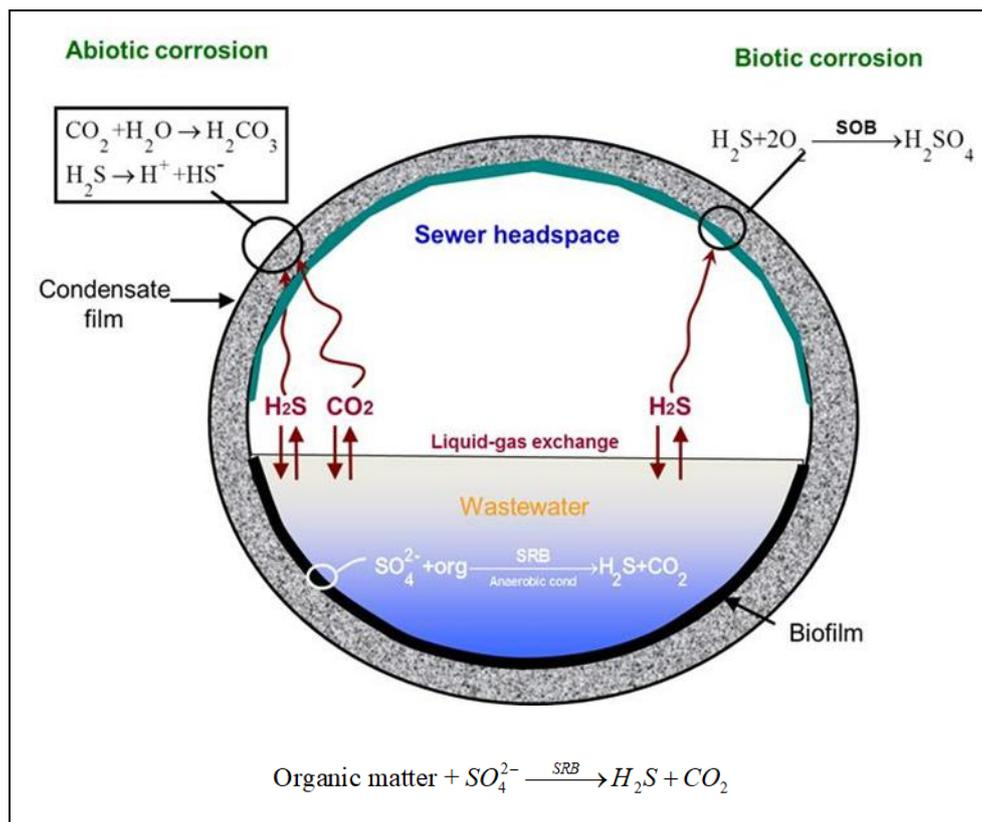
**Figure 5-1 Schematic of sewer processes driving H<sub>2</sub>S and corrosion**
