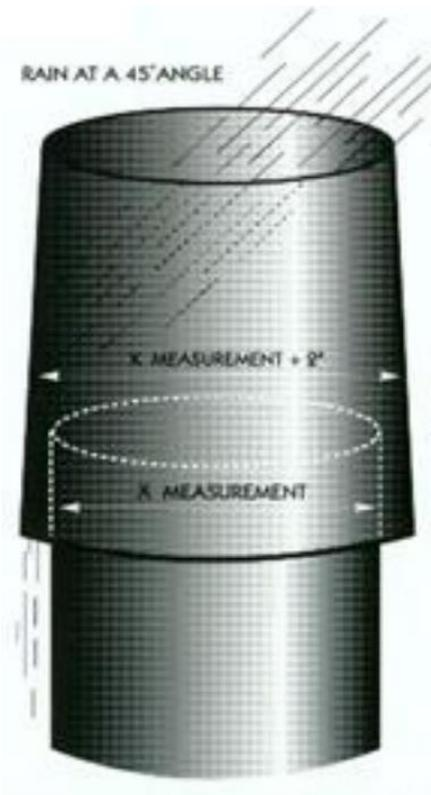
Figure 12-1 Collar-type rain guard for a stack
