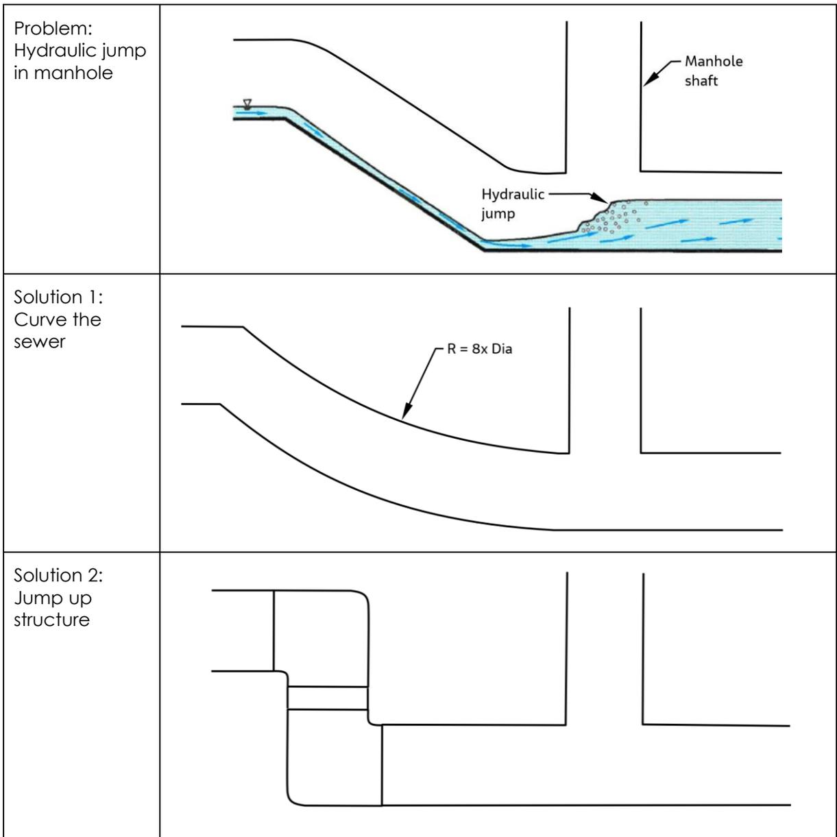
**Figure 7-8 Potential Solutions to a Hydraulic Jump in a Manhole**
