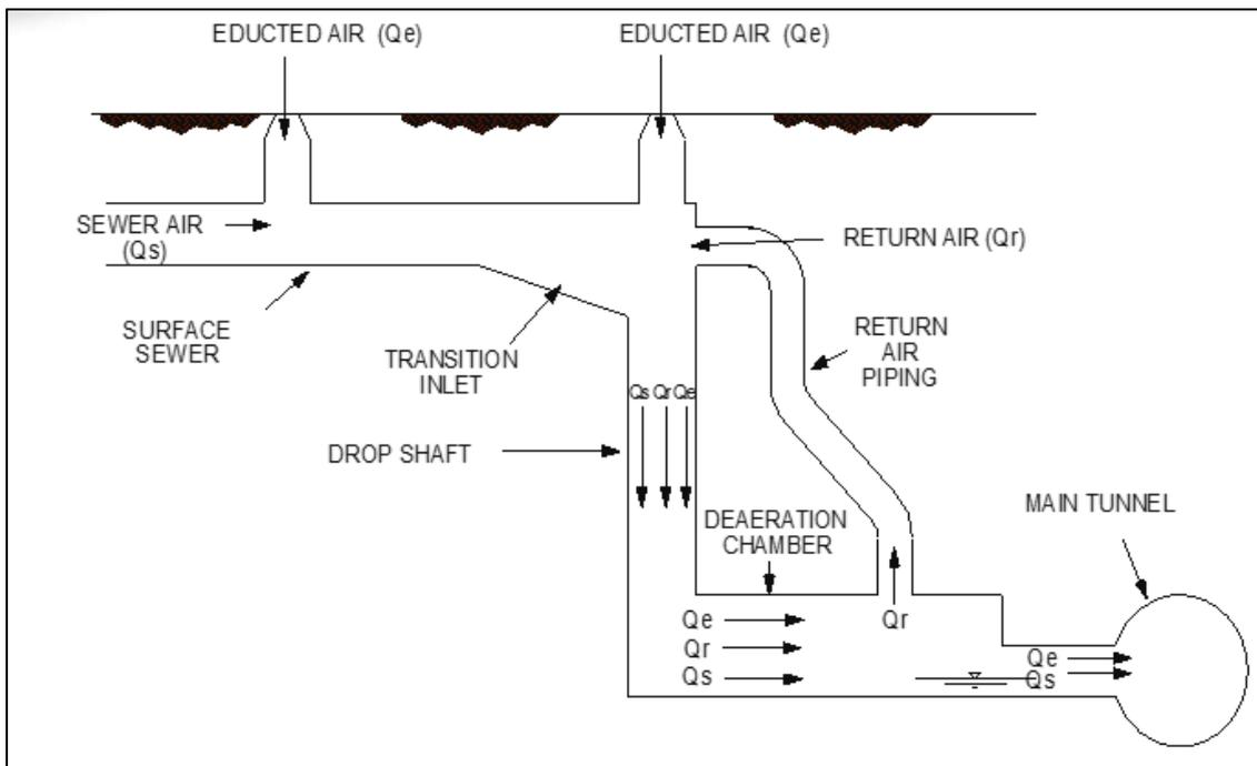
**Figure 6-4 Typical Vortex Dropper with Air Return**
