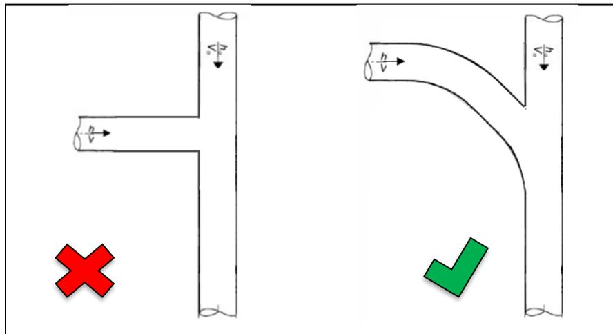
**Figure 7-5 Streamlining branch sewer connections on trunk mains**
