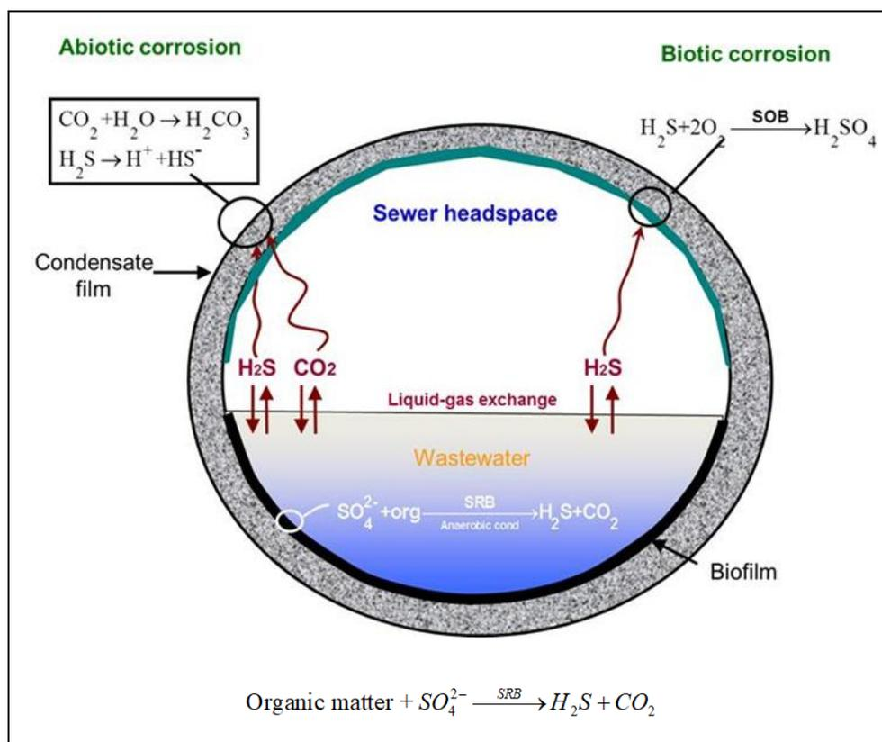
**Figure 5-1 Schematic of sewer processes driving H<sub>2</sub>S and corrosion**
