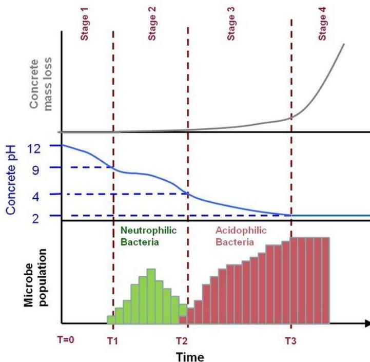
Figure 5-3 Progression of microbial corrosion of sewer pipe
