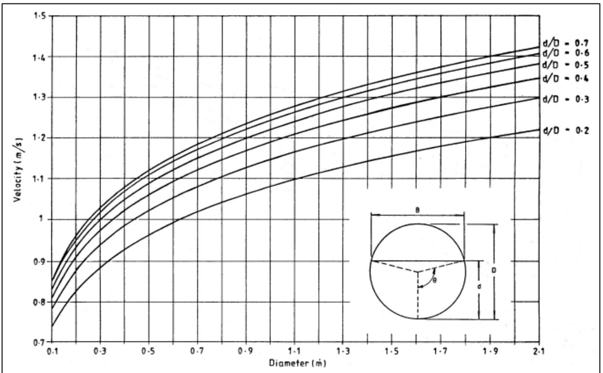
Figure 8-2 Minimum Sewer Velocities for Slime Control [3]
