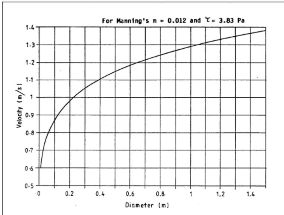
Figure 8-4 Minimum Velocities for Slime Control in Rising Mains [3]
