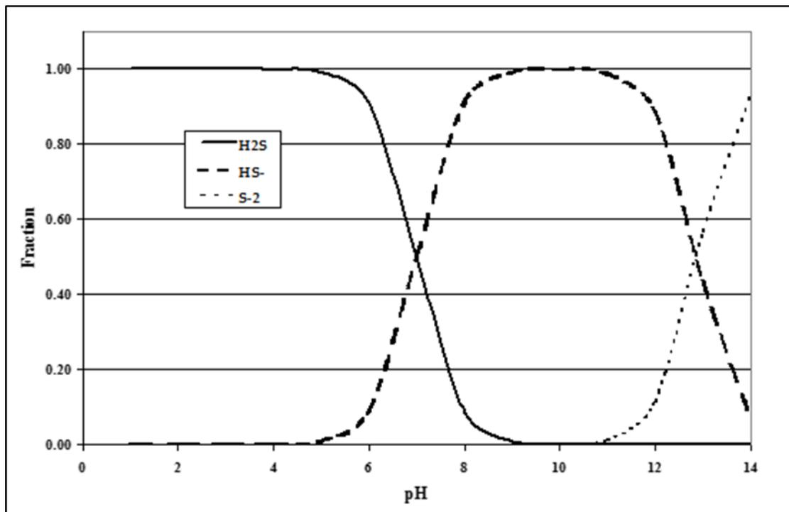
**Figure 5-2 Liquid-Phase Sulphide Distribution vs pH**
