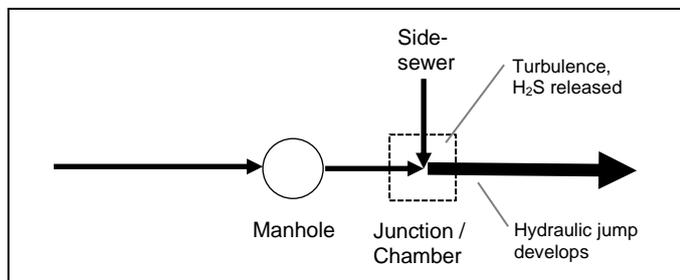
Figure 7-3 Sewer Design to Avoid Hydraulic Jumps
