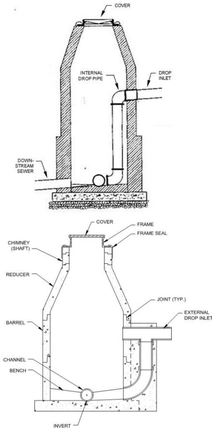
**Figure 6-2 Typical Installations of Hydraulic Drop with Internal and External Drop Pipes**
