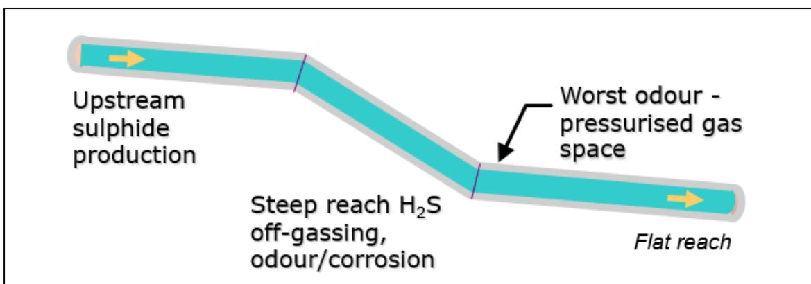
**Figure 7-2 Air Flow Movement at Hydraulic Jump**
