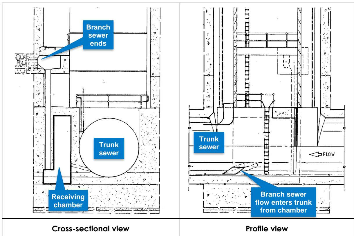
**Figure 7-6 Side chamber for merging flow from branch sewer**
