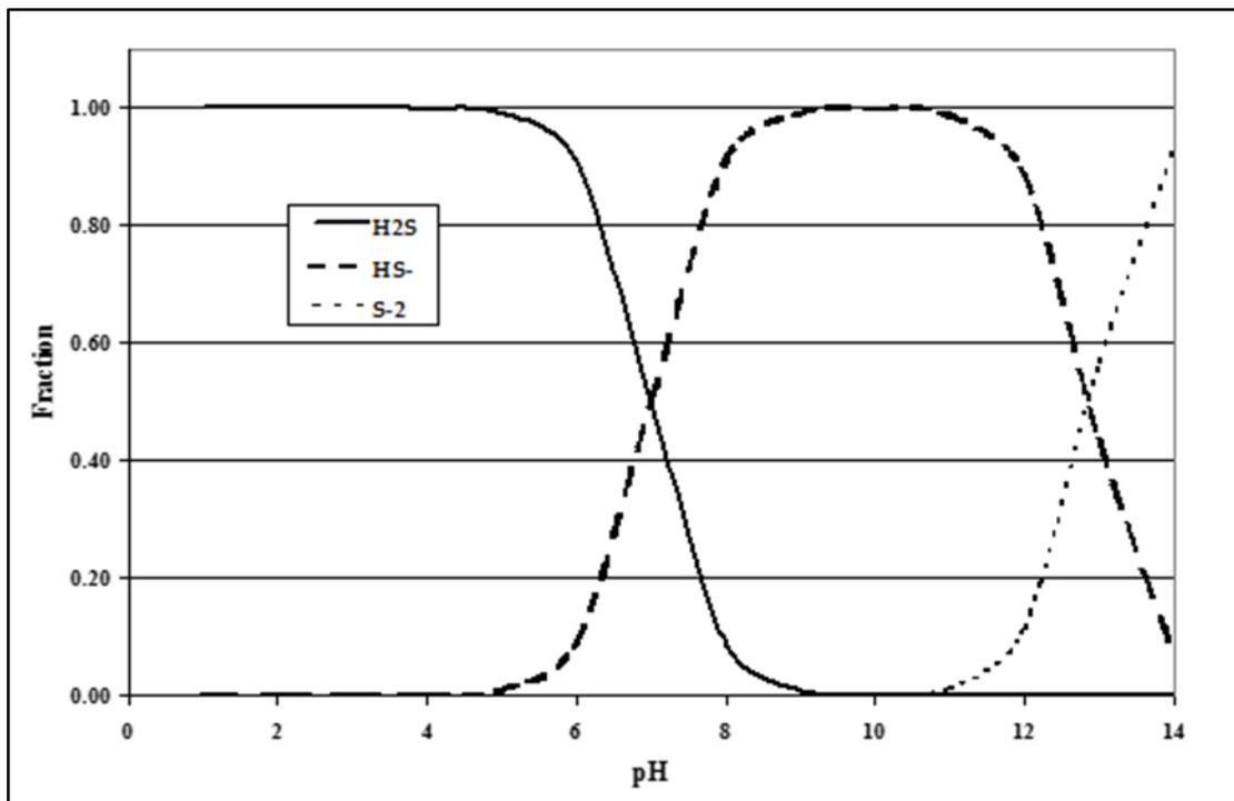
**Figure 5-2 Liquid-Phase Sulphide Distribution vs pH**
