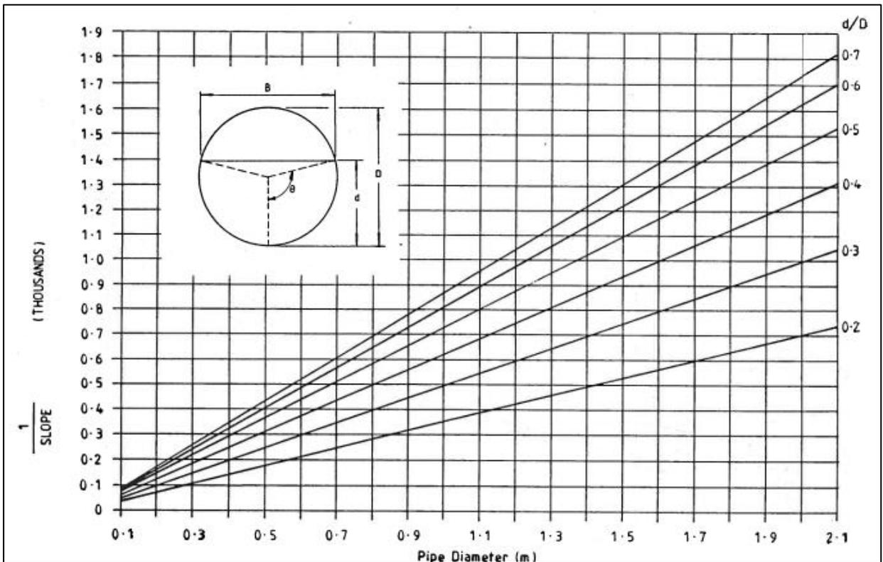
Figure 8-1 Critical Sewer Slopes for Slime Control [3]
