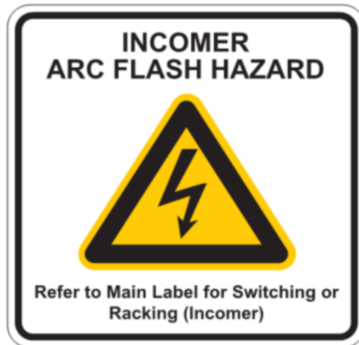
Figure 6-5: Example label to be used where space is limited
