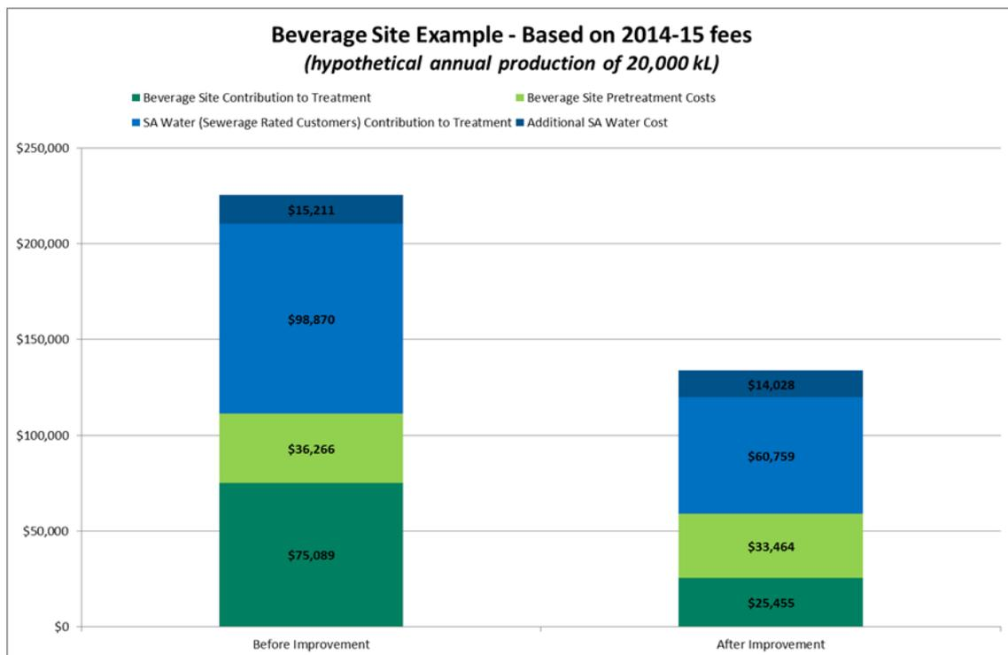
The beverage site example shows that with effective trade waste management, the overall annual cost of associated with the site's trade waste discharge decreased and reduced the cost to SA Water and sewer rate paying customers. The key points are:
