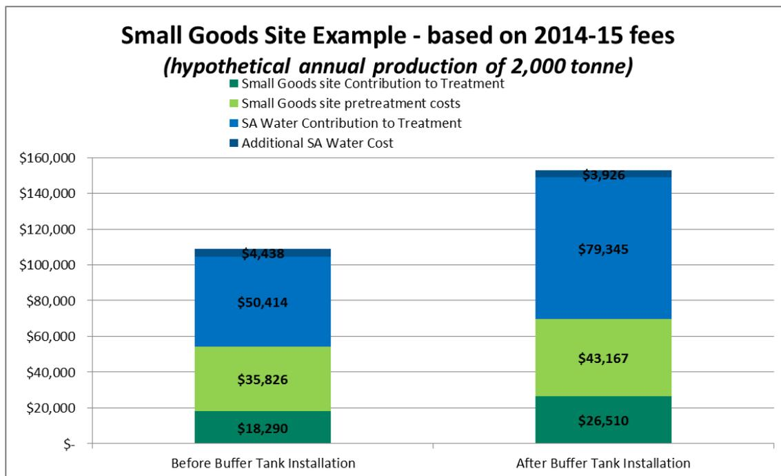
The small goods site example shows that once the buffer tank was installed, the overall cost associated with the site's trade waste discharge increased. The key points are:
