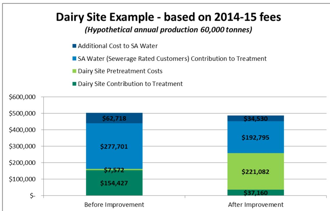
The dairy site example shows that with the installation of a DAF system, the overall annual cost associated with the site's trade waste discharge marginally decreased, but significantly reduced the cost to SA Water and sewer rate paying customers. The key points are:
