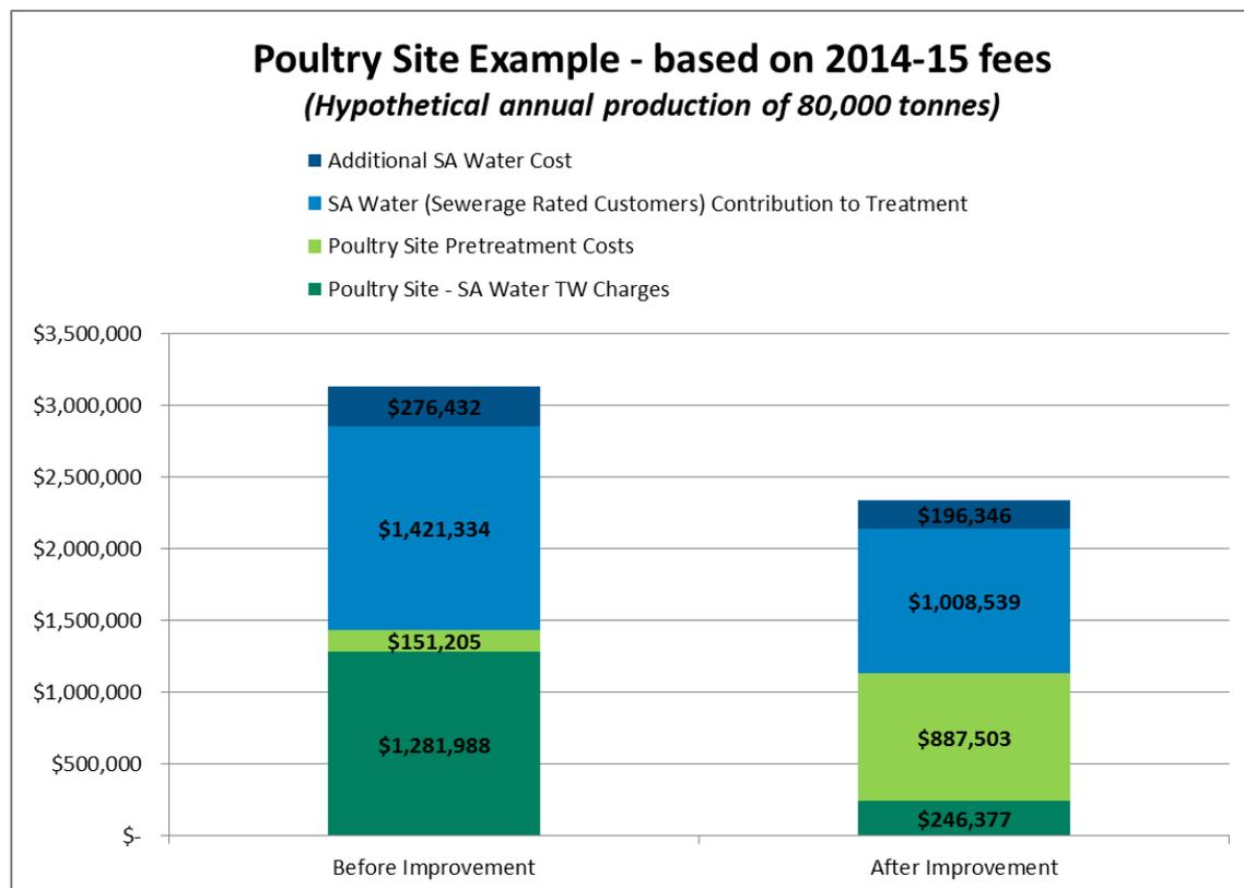
The poultry site example shows that with the installation of a DAF system, the overall annual cost associated with the site's trade waste discharge decreased. The key points are:
