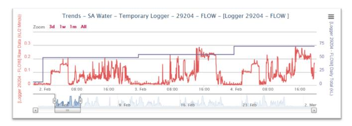
The system has already helped some participating customers to identify leaks and opportunities for improved water efficiency. Through using this type of technology it is not uncommon to identify base flow water use which could be leakage of between 5 and 15 litres per minute.
